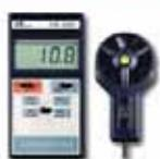
Anemometer – w/Temperature
